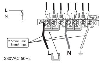
Access to the mains terminal is gained by removing the electrical terminal cover box on the back panel. Connect the mains cable to the correct terminals for your electrical supply type (see fig.). Check that the links are correctly fitted and that the terminal screws are tight. Secure the mains cable using the cable clamp.
